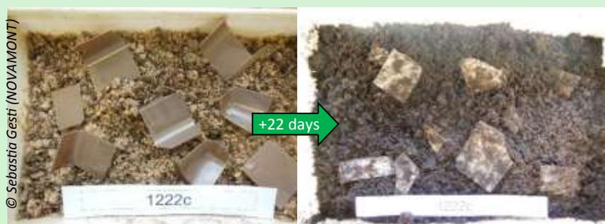
Figure 2: Sample of PHBV+20WSF at the beginning and after 22 days of the test
